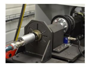
The automobile industry prefers electric motor nut runners for the simple reason that they facilitate the task of logging the date and time of interventions, but for use in other industries, such as wind turbines and notably when a very high torque is required, air motors are nearly always the better choice.
