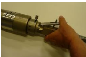
Unlock the safety catch
