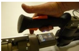
Unlock by pressing the safety trigger
